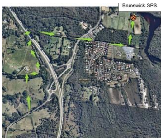
Proposed pressure sewer route layout.
